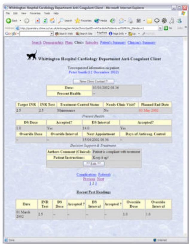
Fig. 5: The “Anticoagulant Application Clinic Contact” screen In the most up-to-date version, HeartBeat, shown in fig. 6, the same decision support engine is used but now accessed via the Web using an “Asynchronous Javascript and XML” (AJAX) technique. As the user fills out the clinic contact pane, they can call for decision support based on values that have already been entered.
