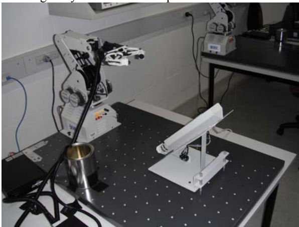
Fig. 7 Lab Volt 5150 robot with mounted gripper setup
