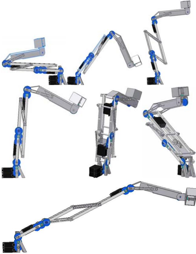
Fig. 3 Multi-joint mechanical arm with five degree of freedom in variety positions
