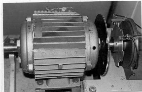
Fig. 1 SR motor with optical head position transducer
