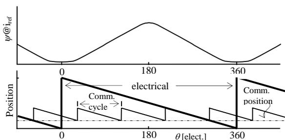
Fig. 4 Position signal definition using constant current
