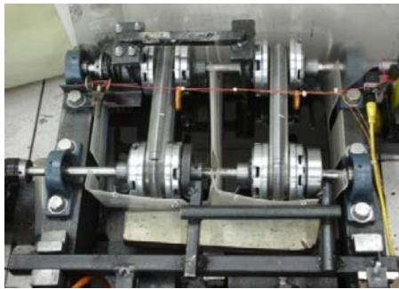
Fig. 6 Prototype of DBCVT and test rig
