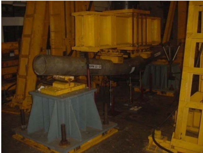
Fig. 2 Close-up view of monotonic fracture experiment
