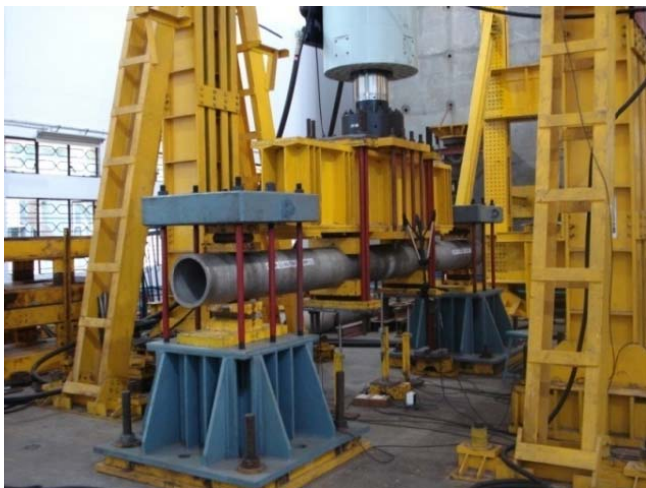
Fig. 3 Close-up view of cyclic fracture experiment
