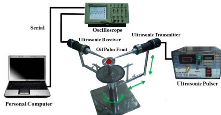
Fig. 1 Ultrasonic experimental setup
