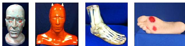
Fig. 1 The four anatomical phantoms used in this investigation (a) polystyrene head mannequin model; (b) plastic radiography head model with 12 traverse slices; (c) a Perspex foot with bone encapsulated; (d) silicone based foot with 3 simulated ulcers
