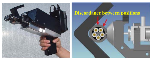
Fig. 3 Cable indenter by KEPRI and its occurred discordance
