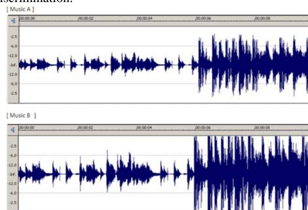
Fig. 2 MusicA and MusicB are same music. Those are converted with different digitalizing standard and different volume level. We can see some points of difference between waveform of two music files
