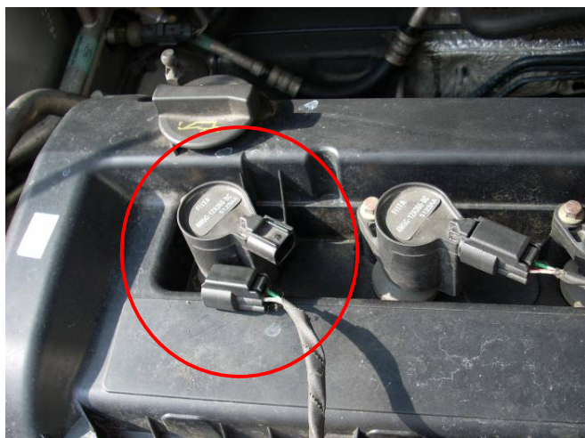
Fig. 10 Offline testing of ignition coil
