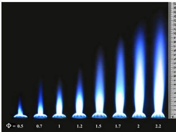
Fig. 9 LPG with 50% Hydrogen IDFs, Re=3000
