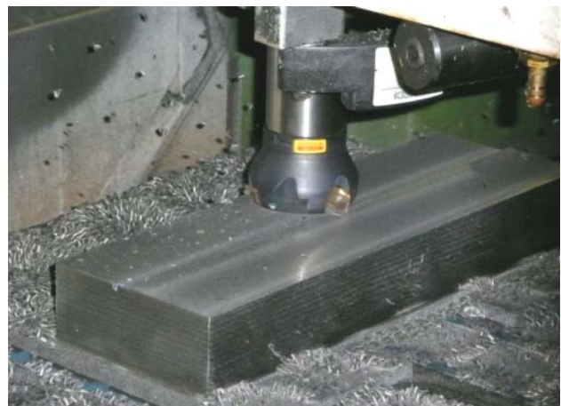
Fig. 2 Magnetic clamping of the workpieces
