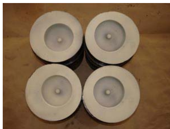
Fig. 3 Photographic View of Piston top (After Ceramic Coating)
