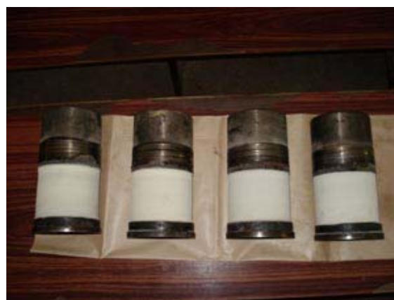
Fig. 2 Photographic View of Cylinder Liner (After Ceramic Coating)
