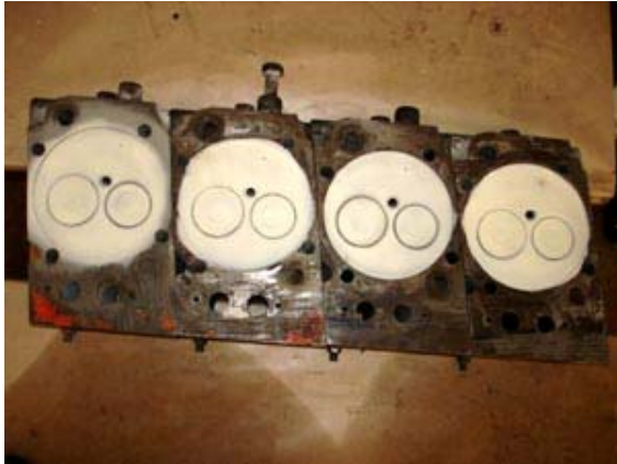
Fig. 4 Photographic View of Cylinder Head with valves (After Ceramic Coating)
