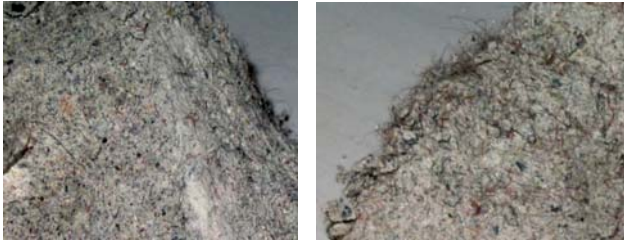
Fig. 5 Propagation of polypropylene fibers in mortar matrix (Left: 0.5% fiber, Right: 1% fiber)
