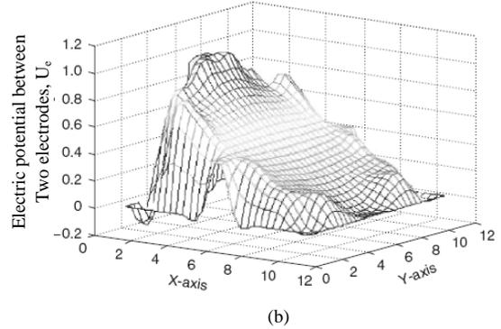
Fig. 7 Distribution of electric potential for fully filled pipe condition
