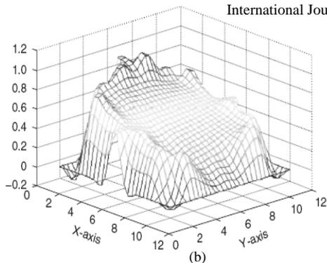
Fig. 8 Distribution of electric potential for 60% filled pipe condition
