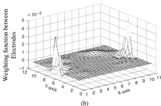
Fig. 9 Distribution of weight function in flow meter for fully filled pipe condition
