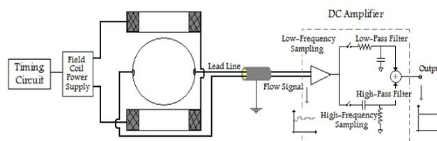
Fig. 3 Signal processing unit
