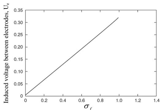
Fig. 11 Induced voltage for constant velocity  $v_m = 2 \frac{m}{s}$
