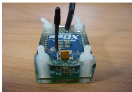
Fig. 1 A sealed but unpackaged STIM transmitter
