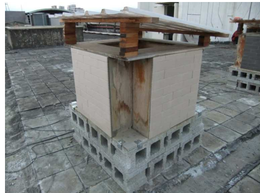
Fig. 5 Experimental group consisting of tiled exterior walls
