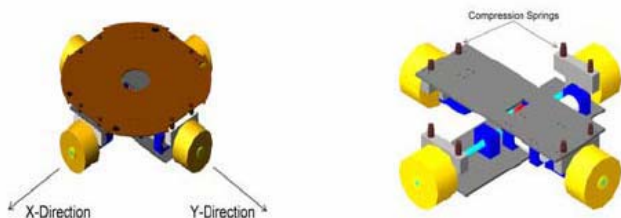
Fig. 2b Left: Robot Navigation System; Each coupled omni wheels provide required acceleration. Relevant vector produces overall acceleration. Right: suspension system for reaching stability
