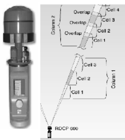
Fig. 6 RDCP600 Doppler current profiler
