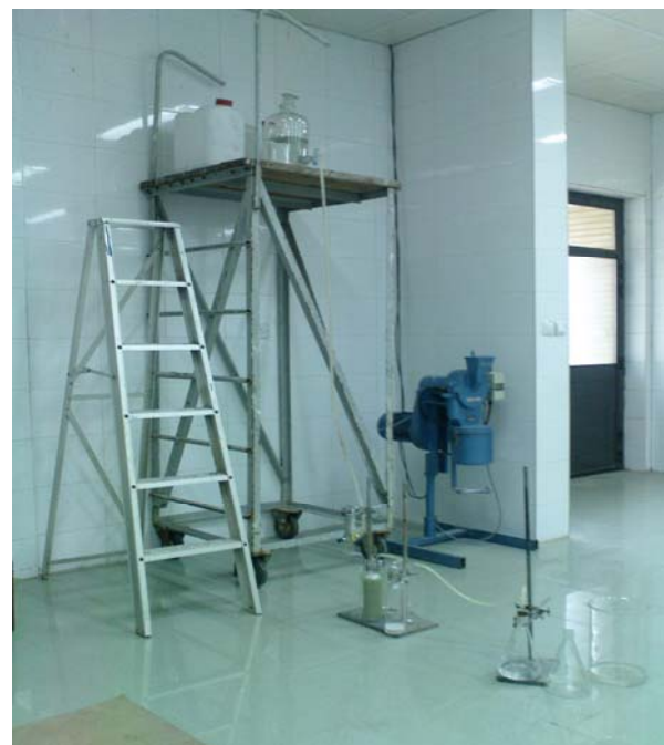
Fig. 1 Experimental set up in column studies
