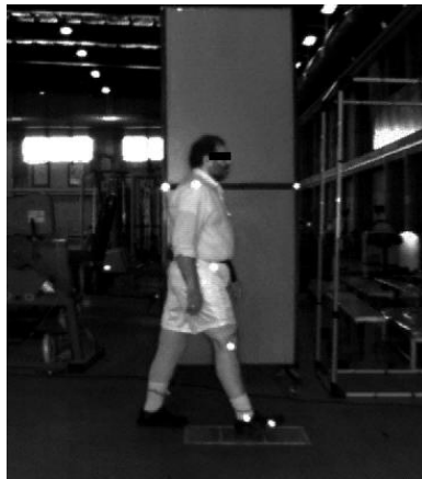
Fig. 1 The locations of markers used in the gait analysis experiment.
