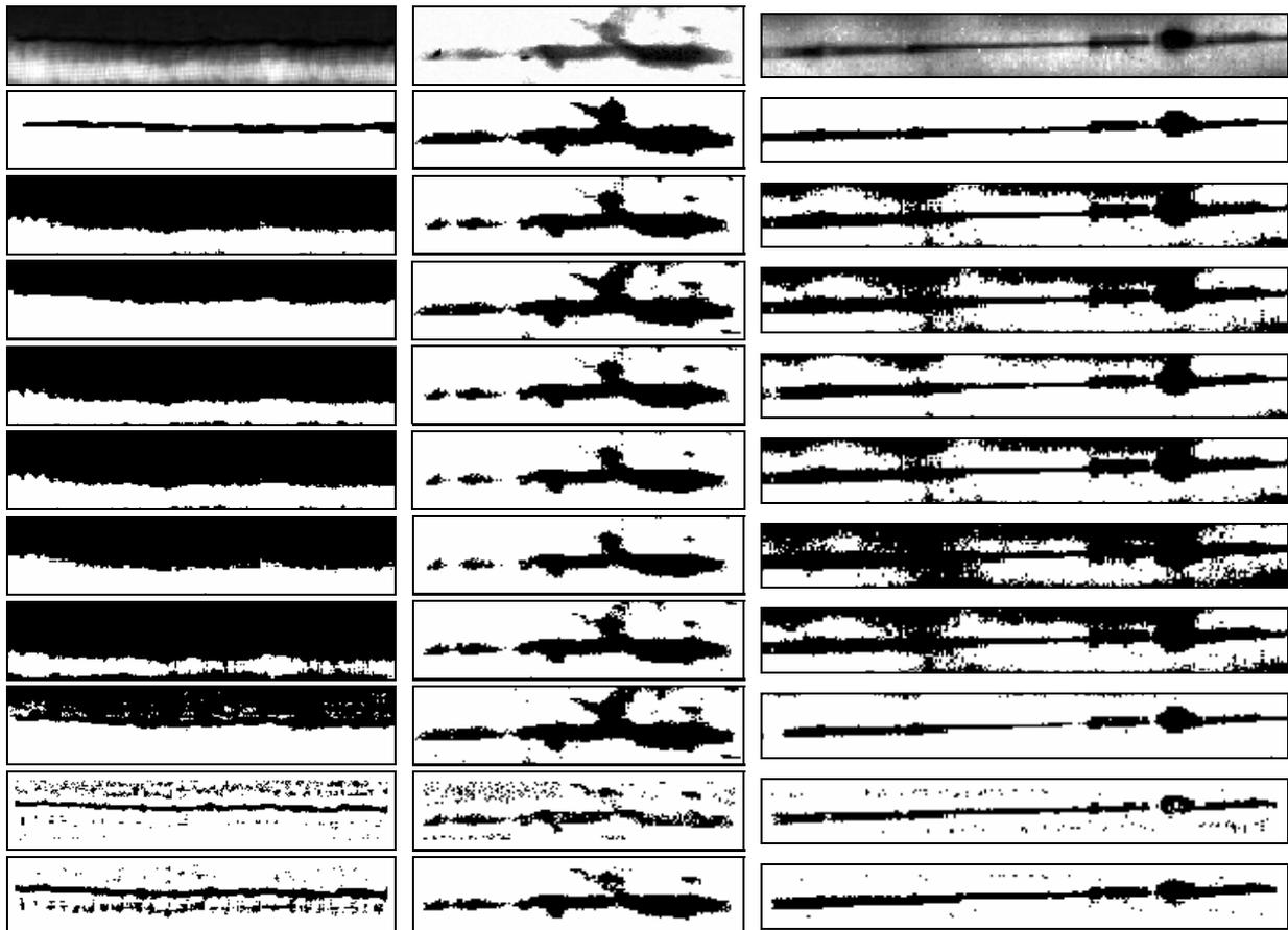
Fig. 3 (from left to right : Images 6 to 8 ) (from top to bottom: Original weld defect image, Ground truth, Thresholding by Otsu, Kittler, Kapur, Tsai, Local entropy, Joint entropy, Relative entropy, Niblack and Sauvola)
