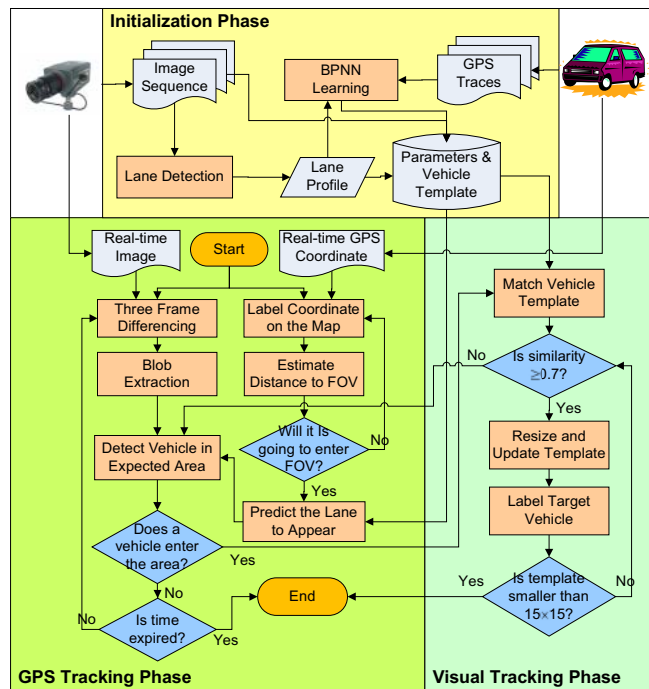
Fig. 3 The operation process of GPS-VT for vehicles
