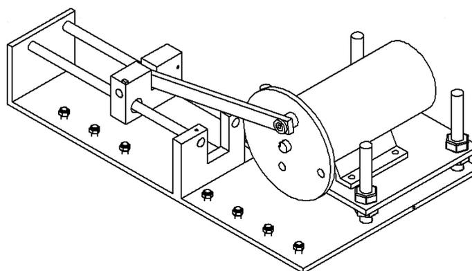
Fig. 13 Mechanism construction: slider – crank mechanism (isometric)
