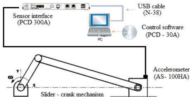
Fig. 14 Scheme of the measuring system
