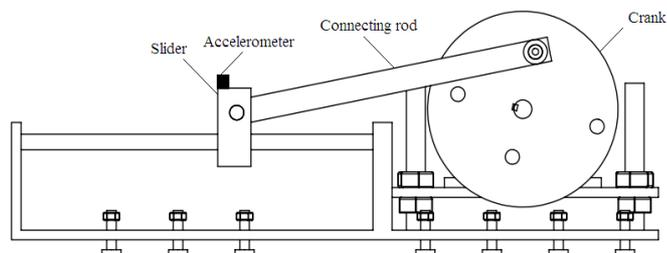
Fig. 12 Mechanism construction: slider – crank mechanism (Front View)
