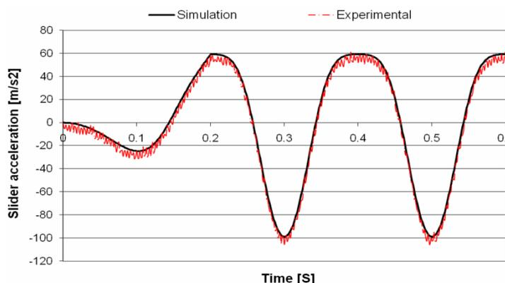
Fig. 15 Simulation and experimentation of slider acceleration in vertical plane at  $\omega = 300$  rpm (without clearance)
