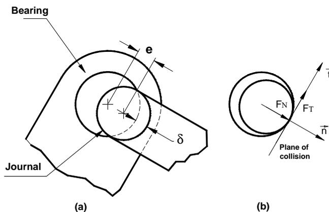
Fig. 1 (a) revolute clearance-joint (b) joint contact forces [13, 14]
