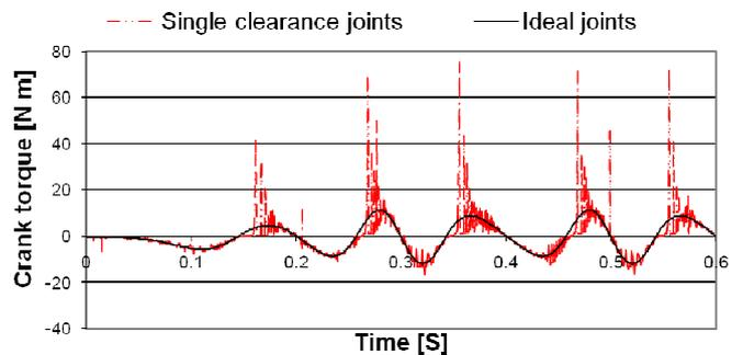
Fig. 9 Applied crank torque at  $\omega = 300$  rpm
