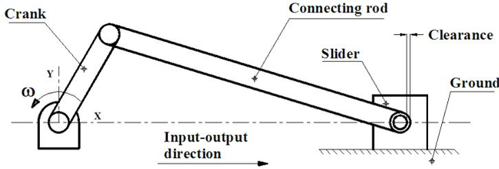
Fig. 5 Slider – crank mechanism with one clearance revolute joint
