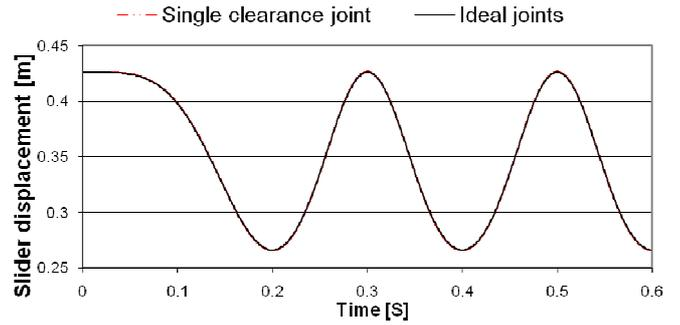
Fig.6 Slider displacement at  $\omega = 300$  rpm
