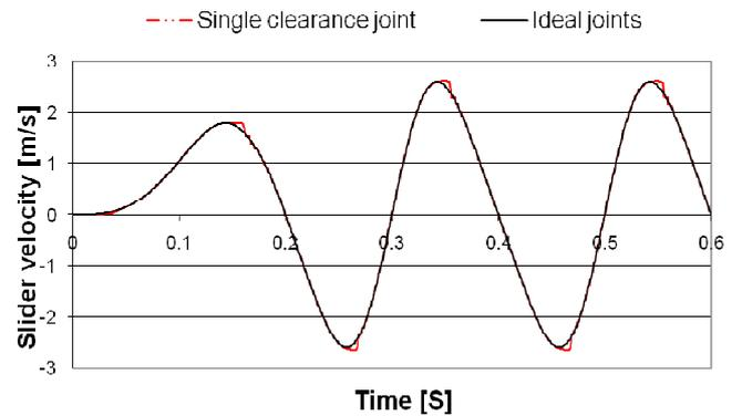
Fig.7 Slider velocity at  $\omega = 300$  rpm
