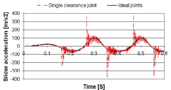
Fig. 8 Slider acceleration at at  $\omega = 300$  rpm
