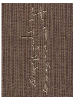
Fig. 4 Original Faulty (Scratch) Fabric
