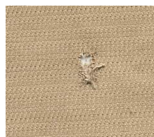
Fig. 6 Original Faulty (Hole) Fabric
