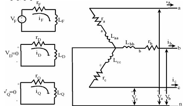
Fig. 2 Schematic diagram of a synchronous generator
