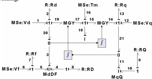
Fig. 3. Bond graph model of a synchronous generator.
