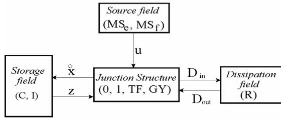
Fig. 1 Key vectors of a bond graph
