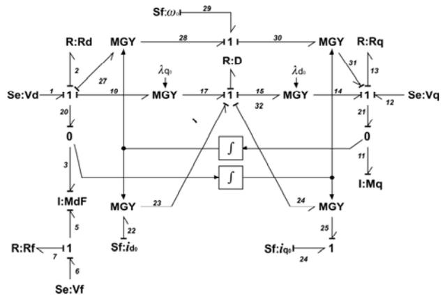
Fig. 5 Bond graph of fast reduced part
