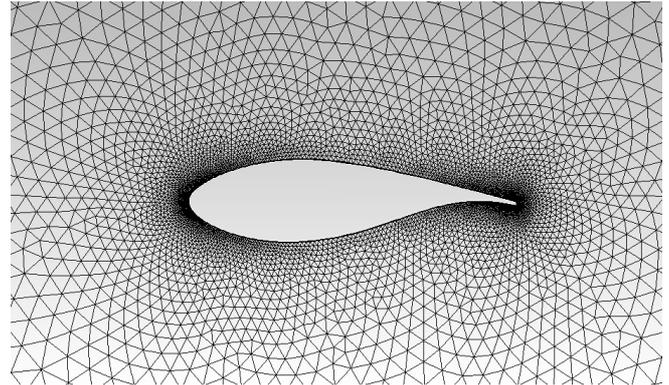
Fig. 8 Airfoil sub-grid mesh, Mod 4
