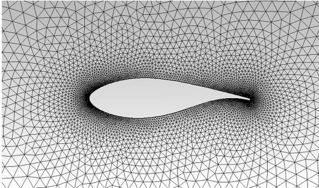
Fig. 5 Airfoil sub-grid mesh, Mod 3
