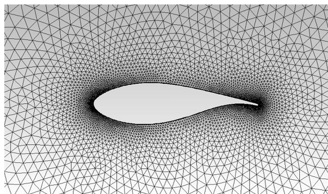
Fig. 4 Airfoil sub-grid mesh, Mod 2
