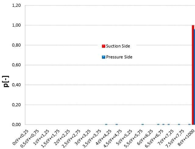
Fig. 13 Graphical representation of the distribution of the  $y^+$  parameter along blade pressure and suction sides; Mod1 mesh,  $\gamma$ - $\theta$  Transitional model
