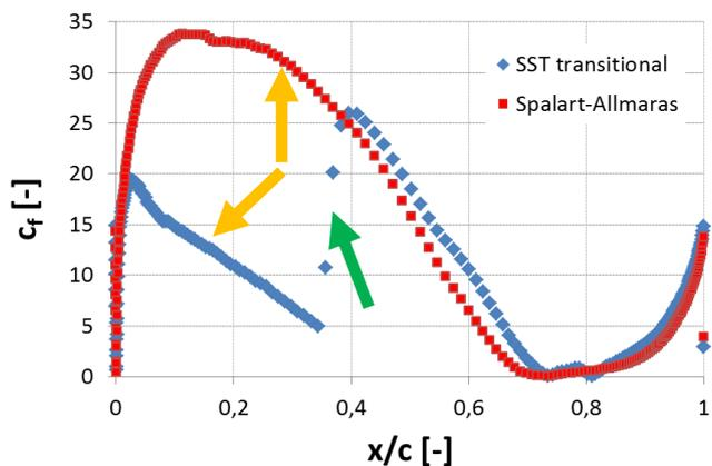
Fig. 18 Numerical predicted skin friction coefficient at pressure side for Mod 3 mesh using both Spalart-Allmaras turbulence model and  $\gamma$ - $\theta$  Transitional model (the green arrow evidences the point of laminar to turbulent transition onset, while the orange arrows evidence the deep differences in skin friction drag prediction between Spalart-Allmaras turbulence model and  $\gamma$ - $\theta$  Transitional model)
