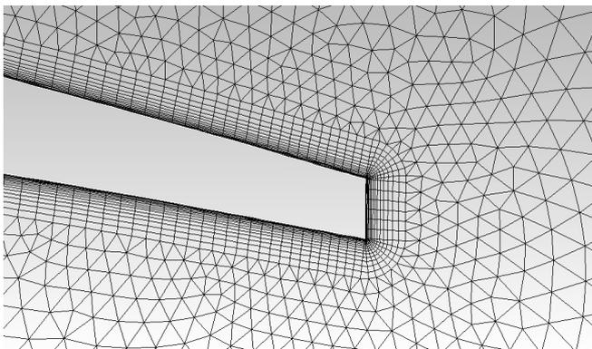
Fig. 7 Trailing edge details of Airfoil sub-grid mesh, Mod 3
