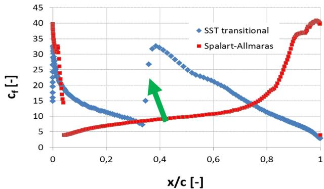
Fig. 17 Numerical predicted skin friction coefficient at suction side for Mod 3 mesh using both Spalart-Allmaras turbulence model and  $\gamma$ - $\theta$  Transitional model (the green arrow evidences the point of laminar to turbulent transition onset)
