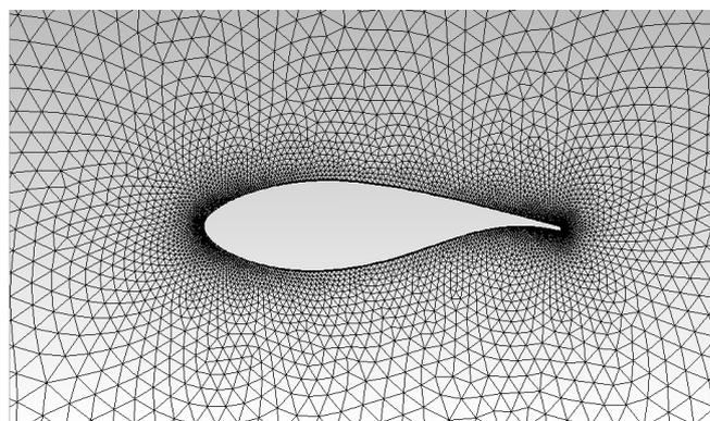
Fig. 3 Airfoil sub-grid mesh, Mod 1
