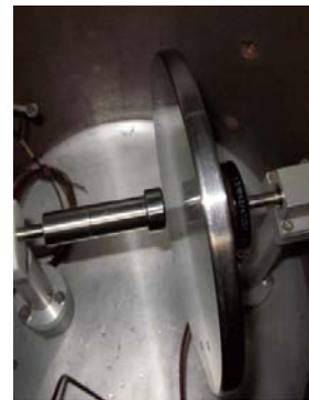
Fig. 2 Stainless Steel electrodes: Rogowski/plane electrode configurations
