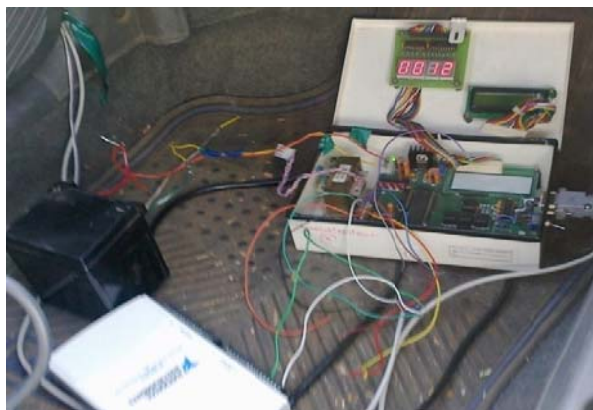
Fig. 8 DAQ card, microcontroller and PC interfacing assembly for speed measurement
