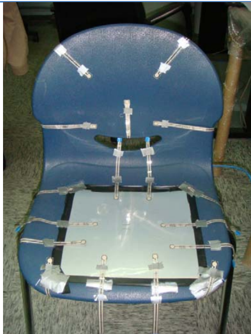
Fig. 5 System with both types of sensors attached. An EMFi sensor and 17 force sensors are shown.
