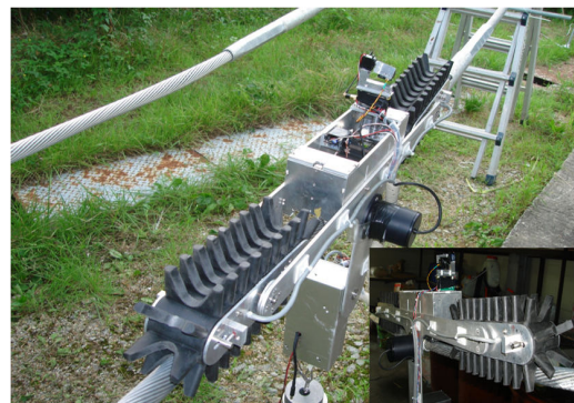
Fig. 10 Mechanical part of line sleeve inspection tool
