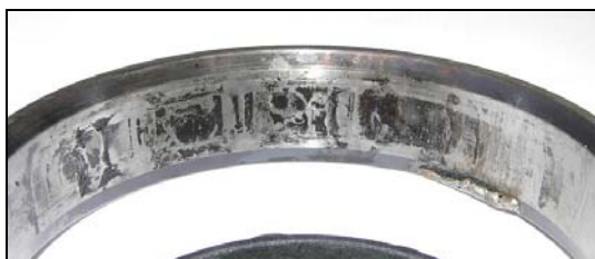
Fig. 14 The defects (dark marks) in the outer race of the bearing
