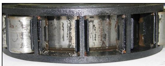
Fig. 15 The defects (dark marks) in the inner race of the bearing
