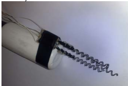
Fig. 10 testing model for multi-flagella propulsion concept
