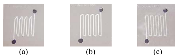
Fig. 2 Flow Patterns in micro PEMFC (a) 30-150, (b)60-120 and (c) 90-90.
