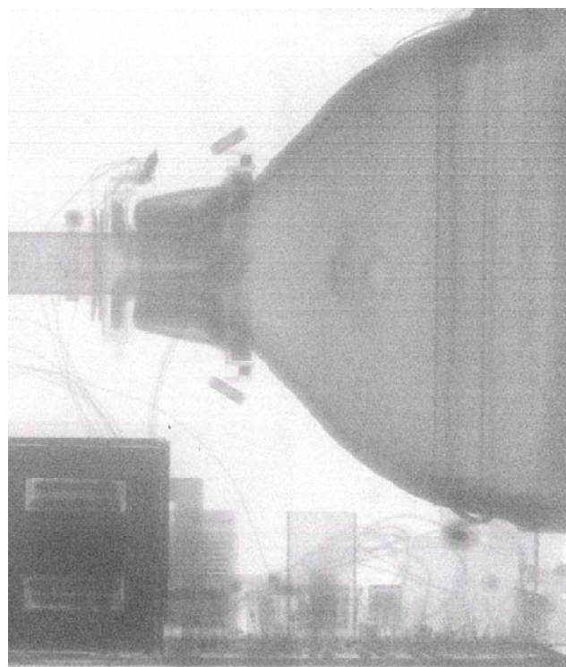
Fig. 3 X-ray radiograph (part of a series for generating a 3D image) of a Cathode Ray Tube (CRT) monitor
