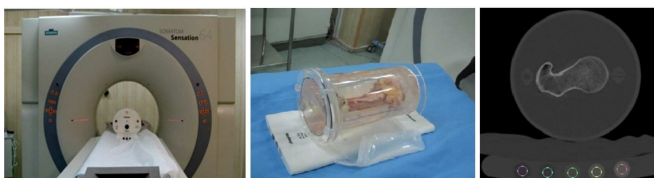
Fig. 3 The CT axial view of the scanner, the imaging and calibration phantoms, and a section of a sample embedded in the imaging phantom
