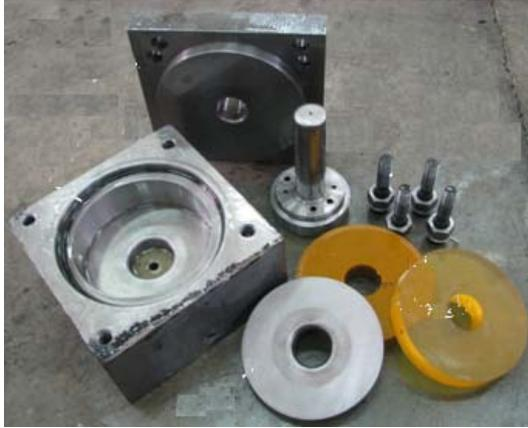
Fig. 2 Photograph of the new die set parts
