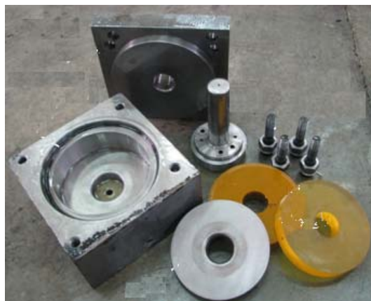
Fig. 2 Photograph of the new die set parts
