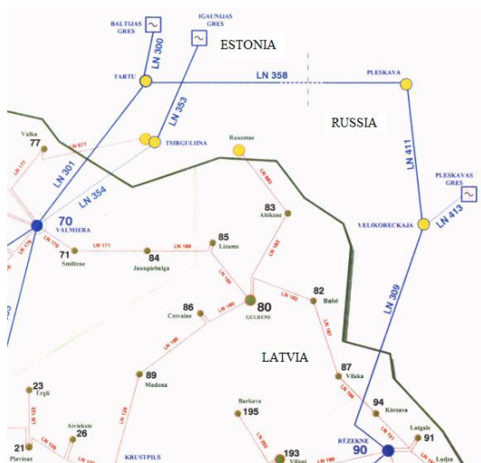
Fig. 1 Part of the electrical diagram of the Latvian power network indicating the location of the existing line "Pleskava-Rezekne"
