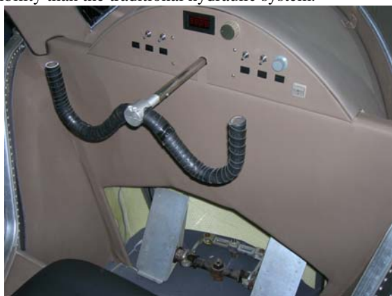
Fig. 6 Real cockpit with control loading system
