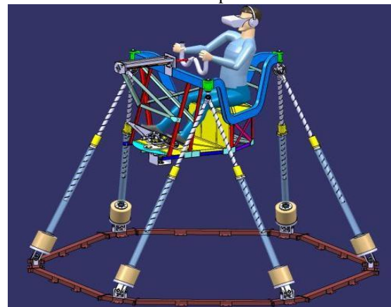
Fig. 3 The low-profile motion platform with subsided cabin
