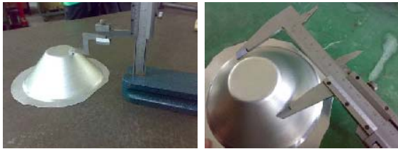
Fig. 6 Diameter measurements along the contour layers
