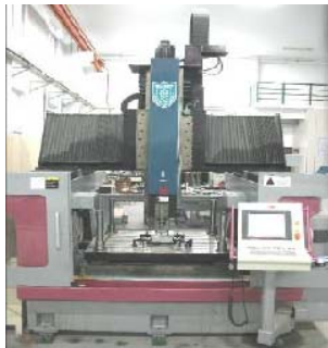
Fig. 3 NC incremental forming machine
