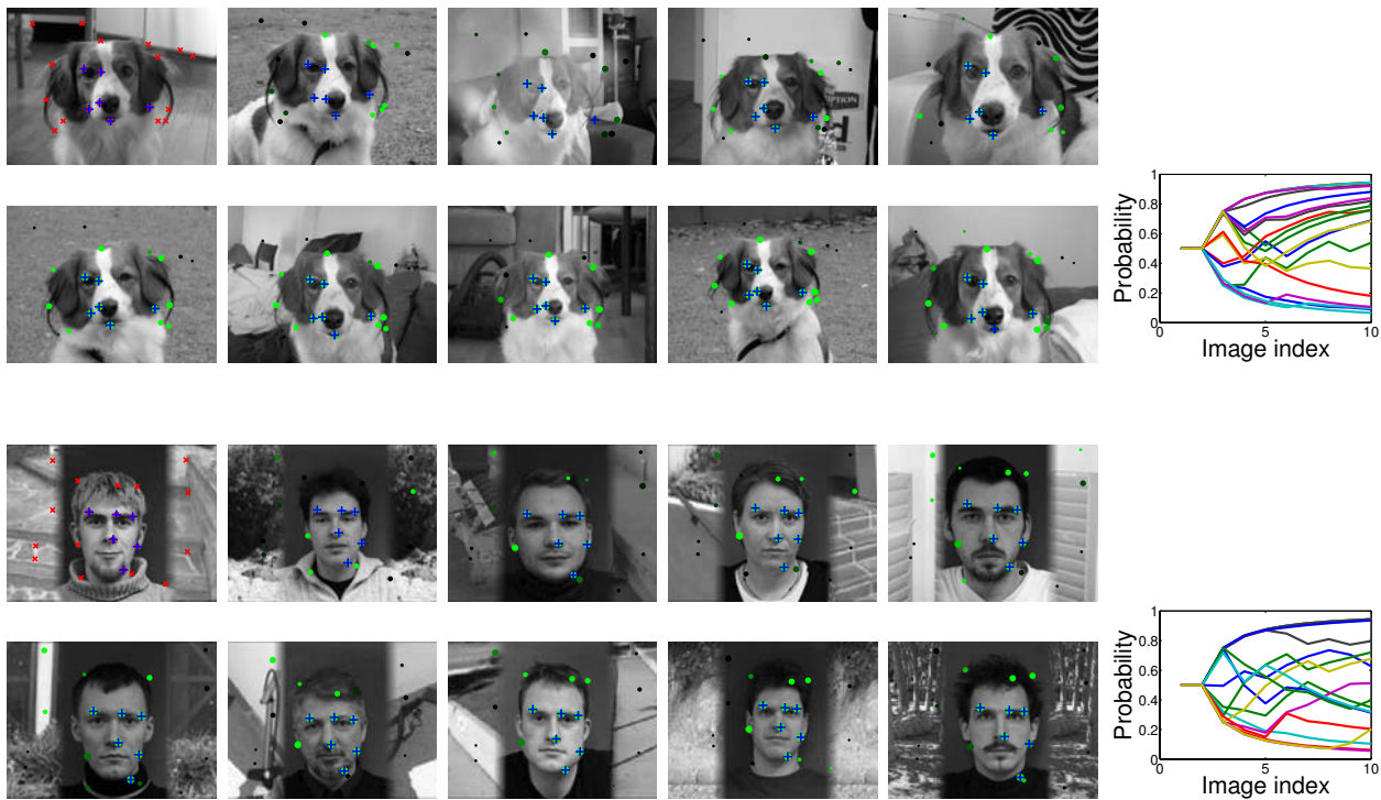
Fig. 4. Two examples of matching sequences of ten images. The dots depict the Monte Carlo estimate of the posterior mean of the node sets. The green values of the dots are proportional to the posterior association probabilities of the nodes. The sizes of the dots are proportional to the prior association probabilities of the nodes which are also shown on the graphs on the right. The nodes whose prior association probability exceeds 0.85 in the end of the sequence are marked with plus signs in the images.
