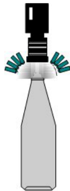
Fig. 4 The illumination of bottle finish
