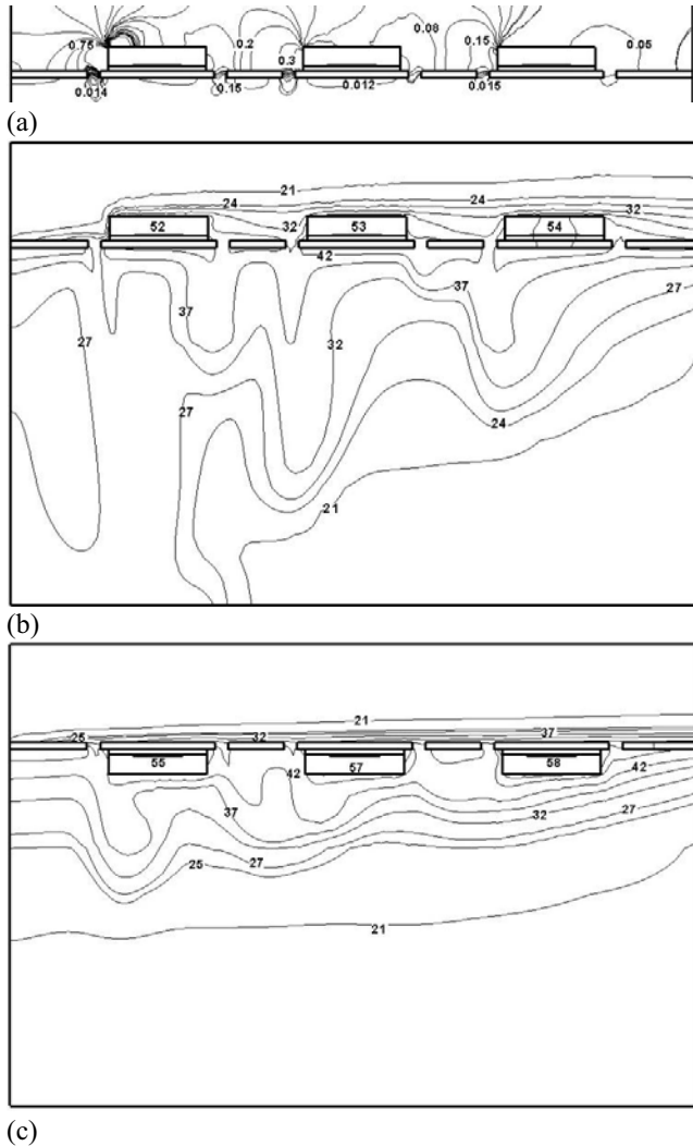
Fig. 9 Temperature distribution of y-z cut plane at the coordinate x at the center of the chips via CFD simulations under forced convection: (a) Case5, pressure distribution near the substrate (face up), (b) Case5, temperature distribution (face up), (c) Case5, temperature distribution (face down)
