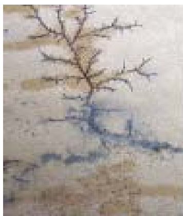
Fig. 3 Case of tracking discharge in wet insulation
