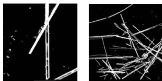
Fig. 2. SEM images of copper nano wires. (bars: 1 \mu m)
