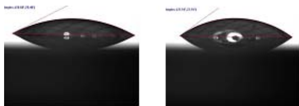
Fig. 13. Surface tension of the solution used for synthesis of copper nanowires (a) before and (b) after the synthesis
