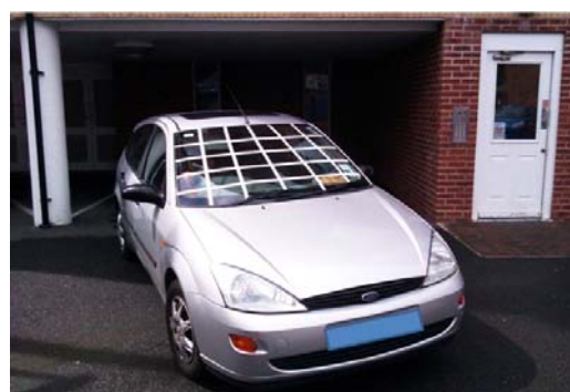
Fig. 1 The windscreen of the Ford Focus car divided into 24 cell
