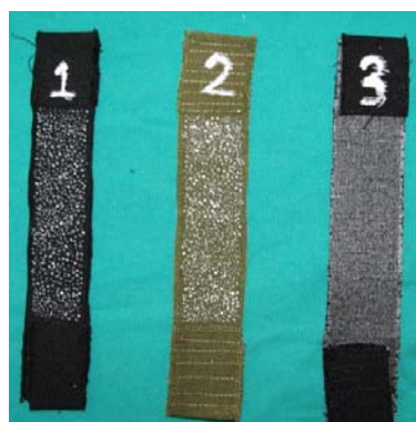
Fig. 1 Example Specimens prepared for uniaxial tensile testing
