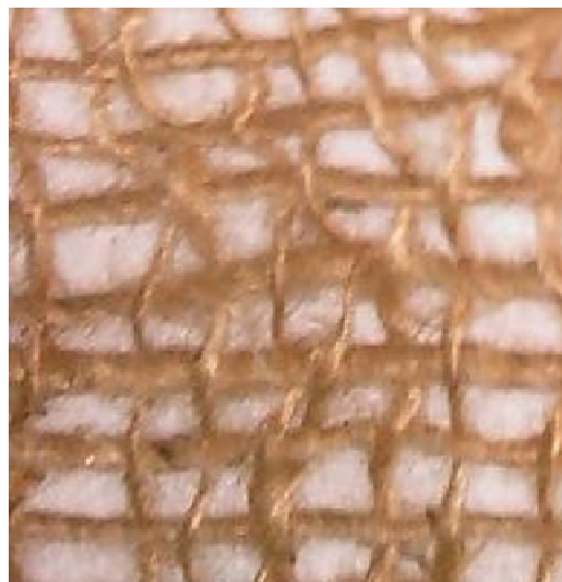
Fig. 5 Photograph of geo-jute used in the field trail of slope protection
