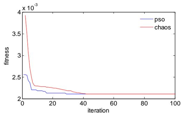
Fig. 6 Convergence of PSO and chaos algorithms
